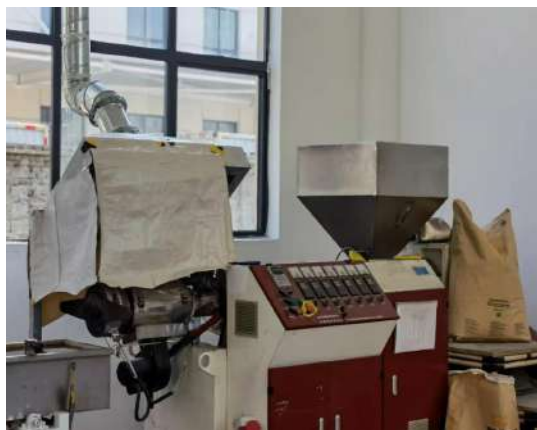
1#辅助车间抽粒废气集气罩
